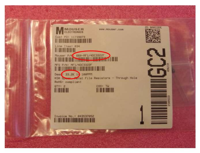
Match the Mouser part number or the description with the parts on the BOM. In this case, you will see that 33.2k resistors are installed at R12 and R15.
